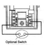
OIn the case there is Negative type output or Relay Output (N.C. or N.O.) from the Control Panel.
