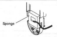
Lead wires through the Wiring Hole on the Unit Base and connect to the terminals. Then, lead wires to the Wiring Groove on the lower side of Unit Base. Be sure to put the wires between sponges on the Unit Base and Back Plate for rain, dust and insect protection.
