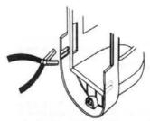
Remove the knockouts for the exposed wiring on one side of the Front Cover with pliers. After wiring, replace the Front Cover on the Unit Base.
