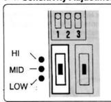
When greater sensitivity is desired, select [H]. When the installation site is poor(bad conditions) select [L].
