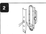
Lead wire through the Wiring Hole on the Unit Base and connect to the terminals. (See Section 6) Be sure to put the wires between sponges on the Unit Base and Back Plate for rain, dust and insect protection.
