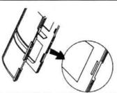
Move the Lens to select the angle (0 or 3 degree) of the detection areas as shown above and confirm that the Lens is unhooked from the groove on the Lens Holder.
