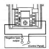
Voltage type > In case there is a programmable (PGM) output terminal (High or Low) from the control panel.
