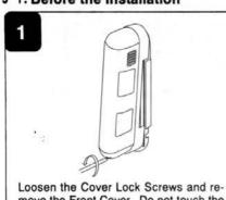
Loosen the Cover Lock Screws and remove the Front Cover. Do not touch the Lens surface.
